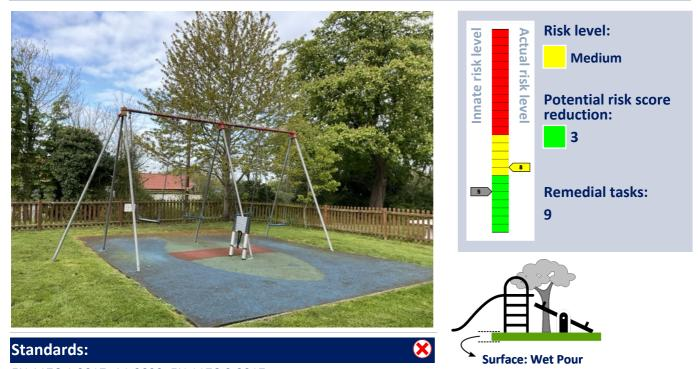
EN 1176-1:2017+A1:2023, EN 1176-2:2017 The item is not compliant with the requirements of the relevant standards. The surfacing meets with the requirements of the relevant standards.
